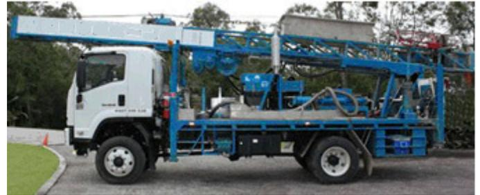
*Typical drilling rig mounted on truck*
