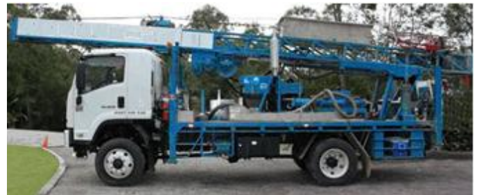
Typical drilling rig mounted on truck
